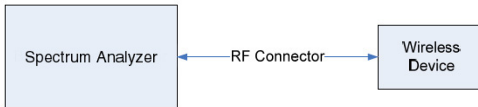
Figure 6-1. WiMAX Conducted Power Test Setup Diagram
