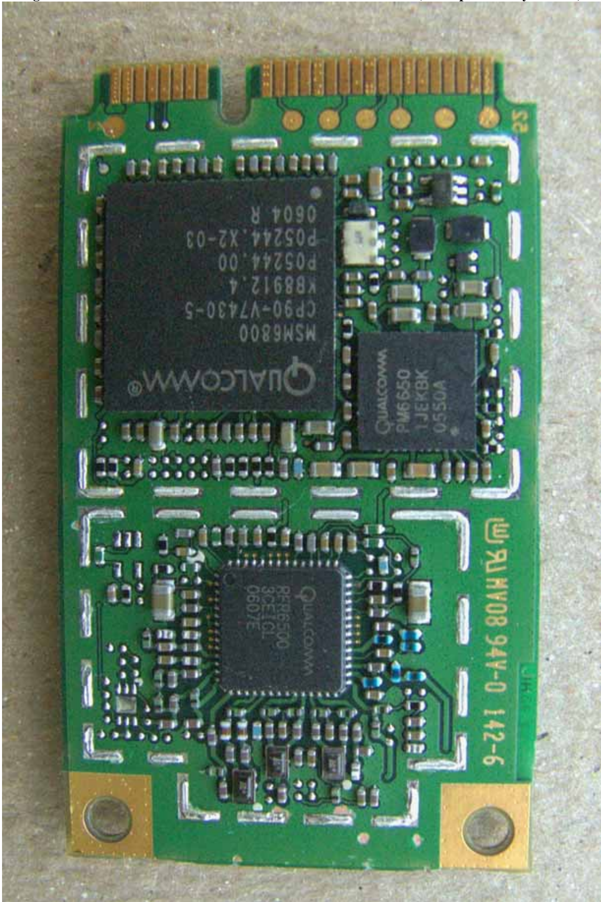
Figure 9: MCD3000 – Bottom of ES720 Radio with Cover Removed (Photo provided by Novatel)
