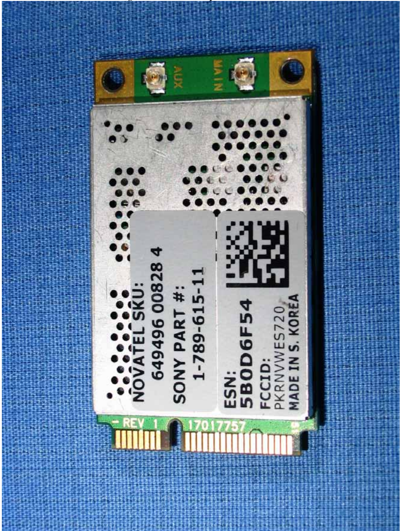
Figure 6: MCD3000 – Top of ES720 Radio
