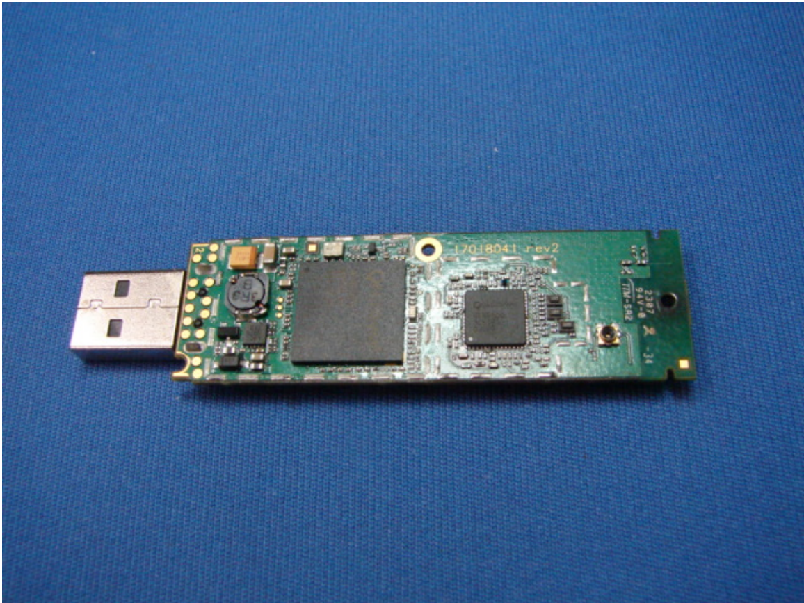
Figure 6: Internal Bare PCB Picture – Bottom
