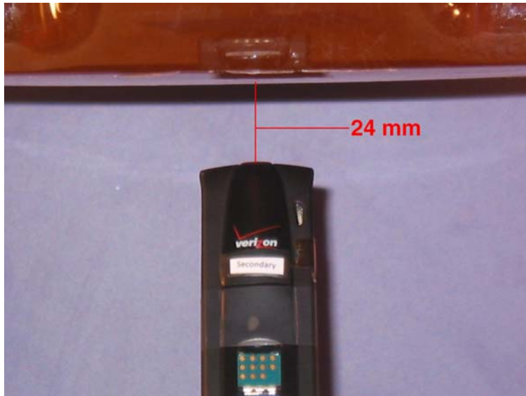
Modem Test Configuration Side E 24 mm Gap
