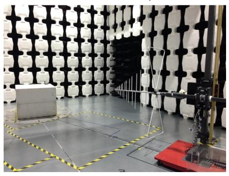
Description: Back view of Radiated Emission Test Setup
