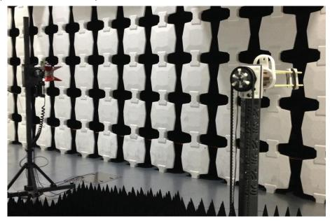
Description: Substitution Antenna for EIRP Test
