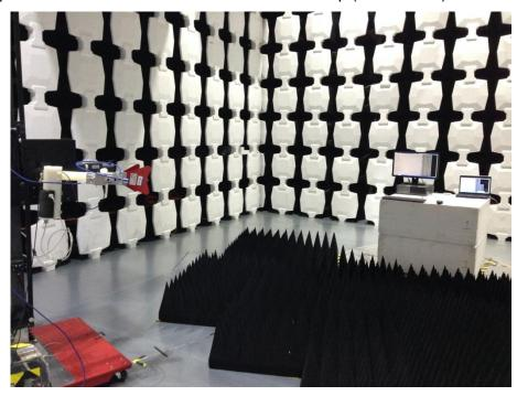
Description: Front view of Radiated Emission Test Setup (30-1000MHz)
