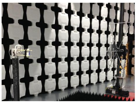
Description: Substitution Antenna for ERP Test
