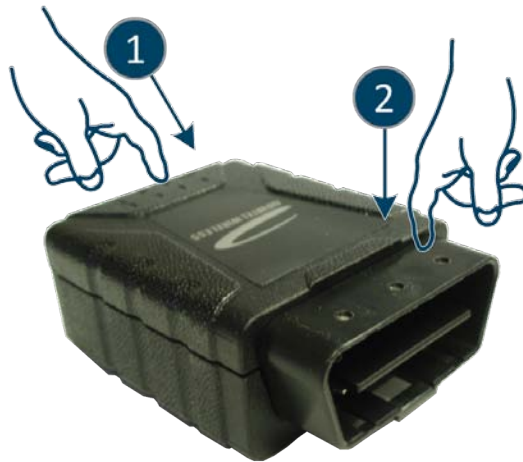
Figure 3-5 MT 3060 Cover Replacement
