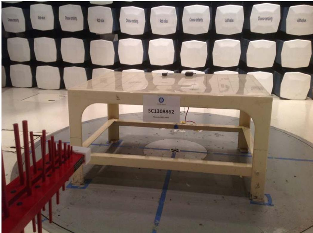
**2.2.11 Test Setup Photo (Below 1GHz Back)**
