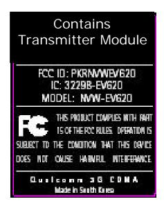
This label must not be stick-on paper label. The label must be permanently affixed to the product and readily visible at the time of purchase and must last the expected lifetime of the equipment and not be readily detached.
