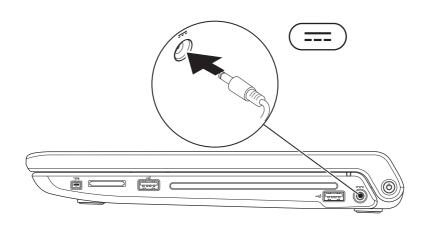
Connect the AC adapter to the computer and then plug it into a wall outlet or surge protector.
