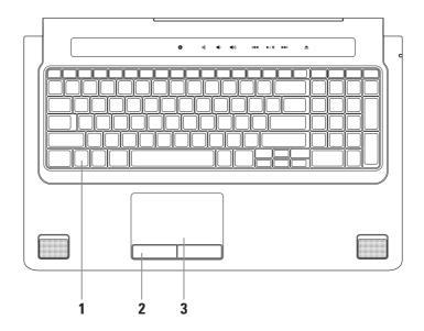
1 Keyboard/Backlit Keyboard (optional) – If you have purchased the optional backlit keyboard, the <F6> key has the backlit keyboard icon \*\*\*\* on it. The optional backlit keyboard provides visibility in dark environments by illuminating all symbols on the keys.
