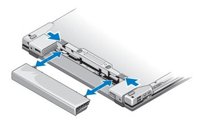
Remove the battery by sliding the battery tabs inward and move the battery away from the notebook. Install the battery by pushing the battery inward until it clicks into place.
