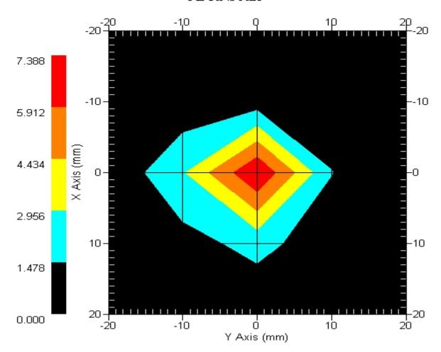
1 gram SAR value : 5.892 W/kg 10 gram SAR value : 1.505 W/kg Area Scan Peak SAR : 7.388 W/kg Zoom Scan Peak SAR : 19.315 W/kg
