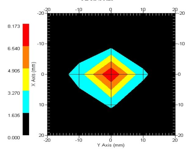
1 gram SAR value : 6.298 W/kg 10 gram SAR value : 1.544 W/kg Area Scan Peak SAR : 8.173 W/kg Zoom Scan Peak SAR : 21.817 W/kg
