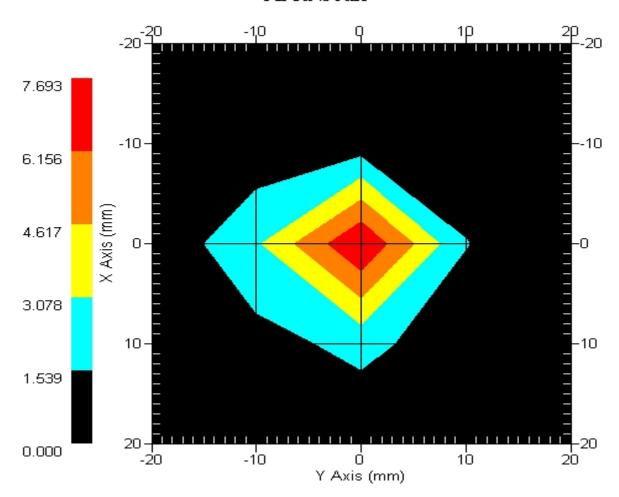
1 gram SAR value : 5.992 W/kg 10 gram SAR value : 1.530 W/kg Area Scan Peak SAR : 7.693 W/kg Zoom Scan Peak SAR : 19.415 W/kg
