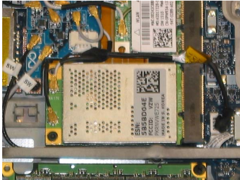
RF Modules Installed
