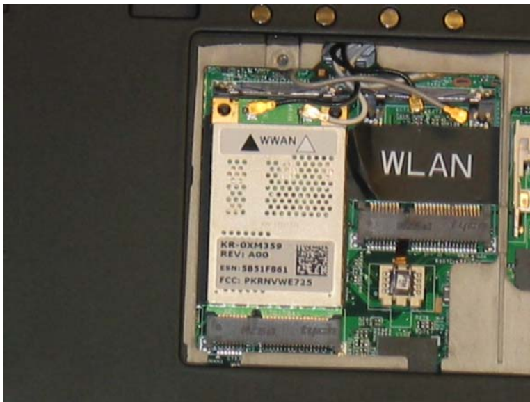
RF Module Installed
