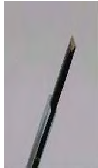
EX3DV4 E-Field Probe
