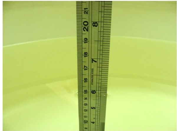
Fig 6.2 Photo of Liquid Height for Body SAR
