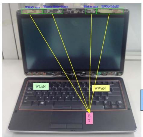
WWAN Main to BT 303mm WWAN Aux to BT 330mm WLAN Main to BT 308mm WLAN Aux to BT 295mm
