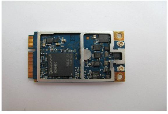
Internal of EUT – 4 (WWAN Module)
