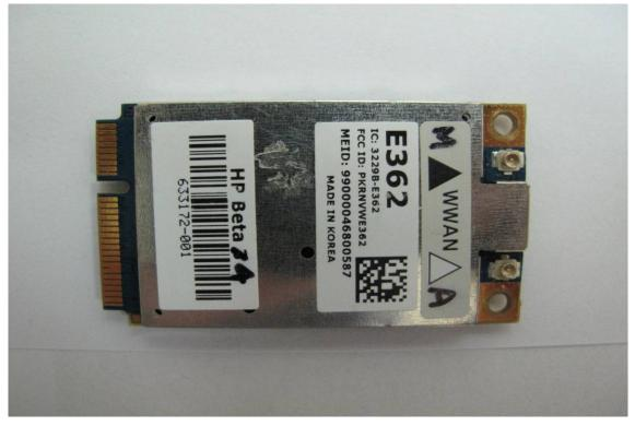
Internal of EUT – 2 (WWAN Module)
