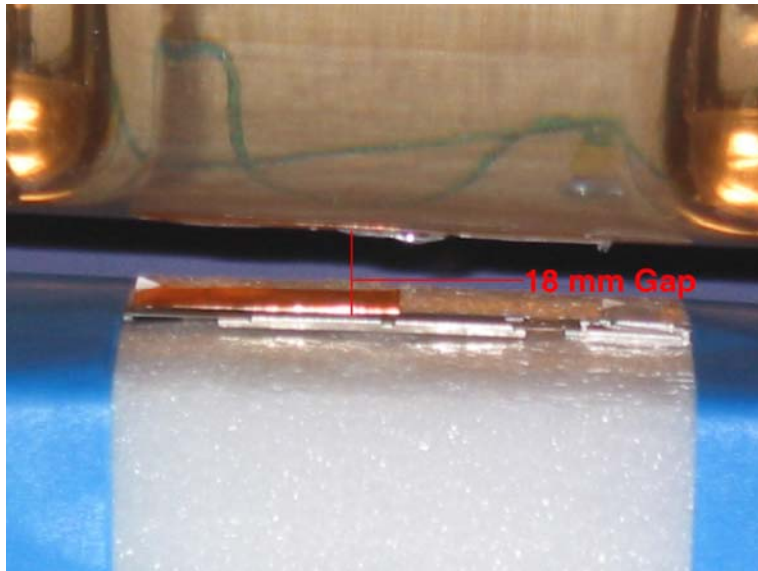
Antenna Test Configuration Side A 18 mm Gap
