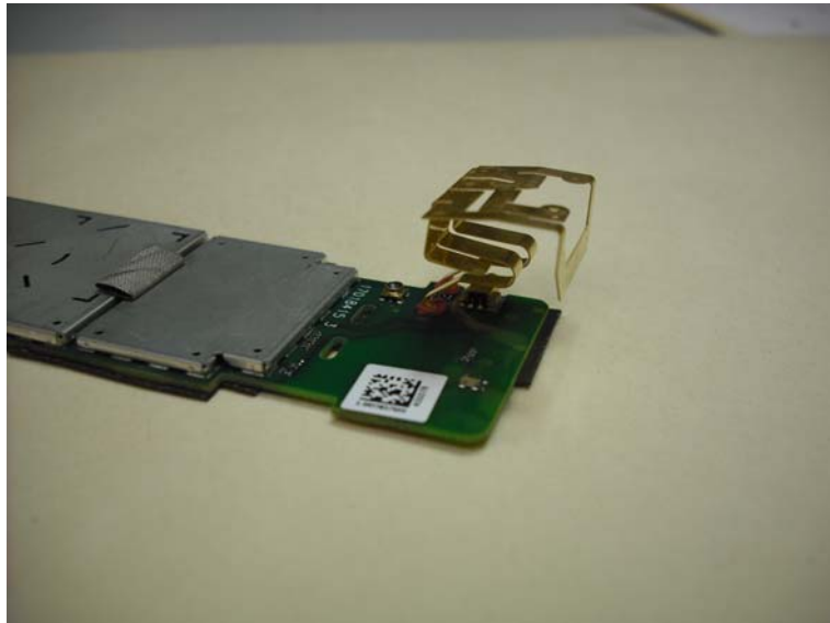
Antenna Mounted on PCB with Clay for Picture Only. Antenna is normally compression contact.
