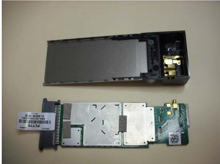
Front of PCB With Front Cover Removed Antenna Installed In Cover
