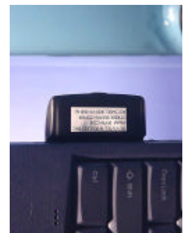
Body SAR Test Setup 1.5cm Separation Distance
