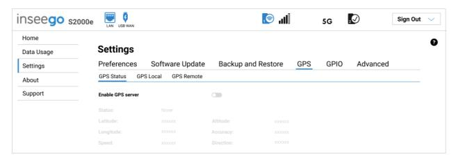
**Enable GPS server:** This setting enables or disables the GPS radio on your S2000e. When the **ON/OFF** slider is **ON**, the device acquires GPS and makes GPS location data available on this page. A GPS Agreement appears, click **Confirm** to proceed. When **OFF**, no GPS data is available.
