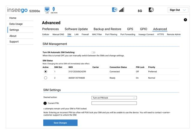
**NOTE:** The SIM card in your S2000e can be locked using a PIN. If the SIM card is locked, you must enter the PIN before connecting to the mobile network. Once entered, the PIN is remembered until the next shutdown. You may also need to provide the existing PIN to change a SIM. The default PIN is available from your service provider.
