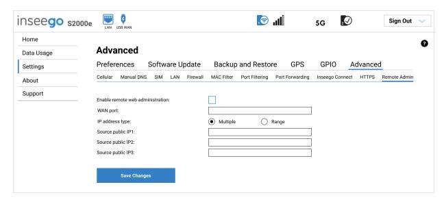
**Enable remote web administration:** To enable remote web administration, move the **ON/OFF** slider to **ON**. To disable remote web administration, move the **ON/OFF** slider to **OFF**.
