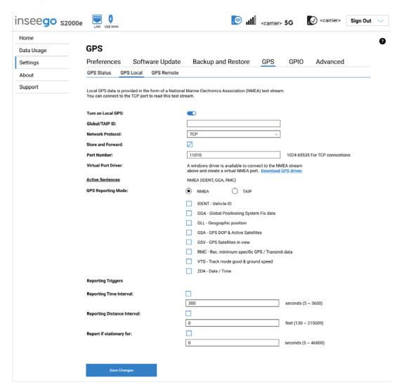
**Turn on Local GPS:** Check this box to turn on GPS streaming on the local network.
