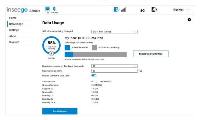
**SIM information being displayed:** Use the drop-down to change the SIM on which data usage is displayed.
