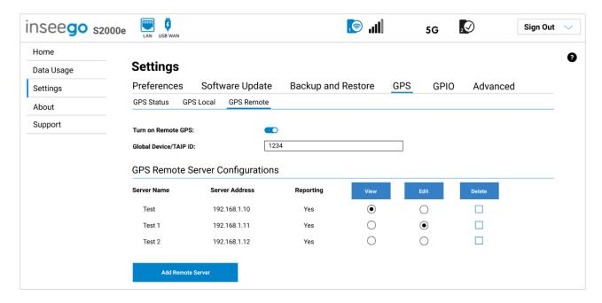
**Turn on Remote GPS:** Check this box to turn on GPS streaming to remote servers.
