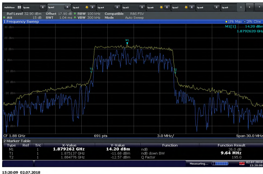
CA_2A-13A_10+10 MHz Bandwidth_PCC_Band 2_1880 MHz_QPSK / 26dB BW
