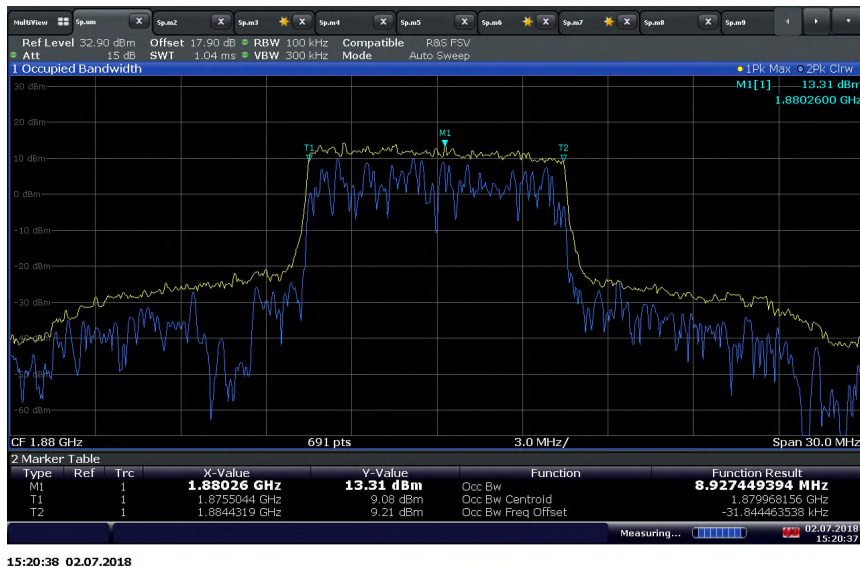
CA_2A-13A_10+10 MHz Bandwidth_PCC_Band 2_1880 MHz_QPSK / 26dB BW
