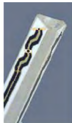
Figure 2.3 Probe Thick-Film Technique
