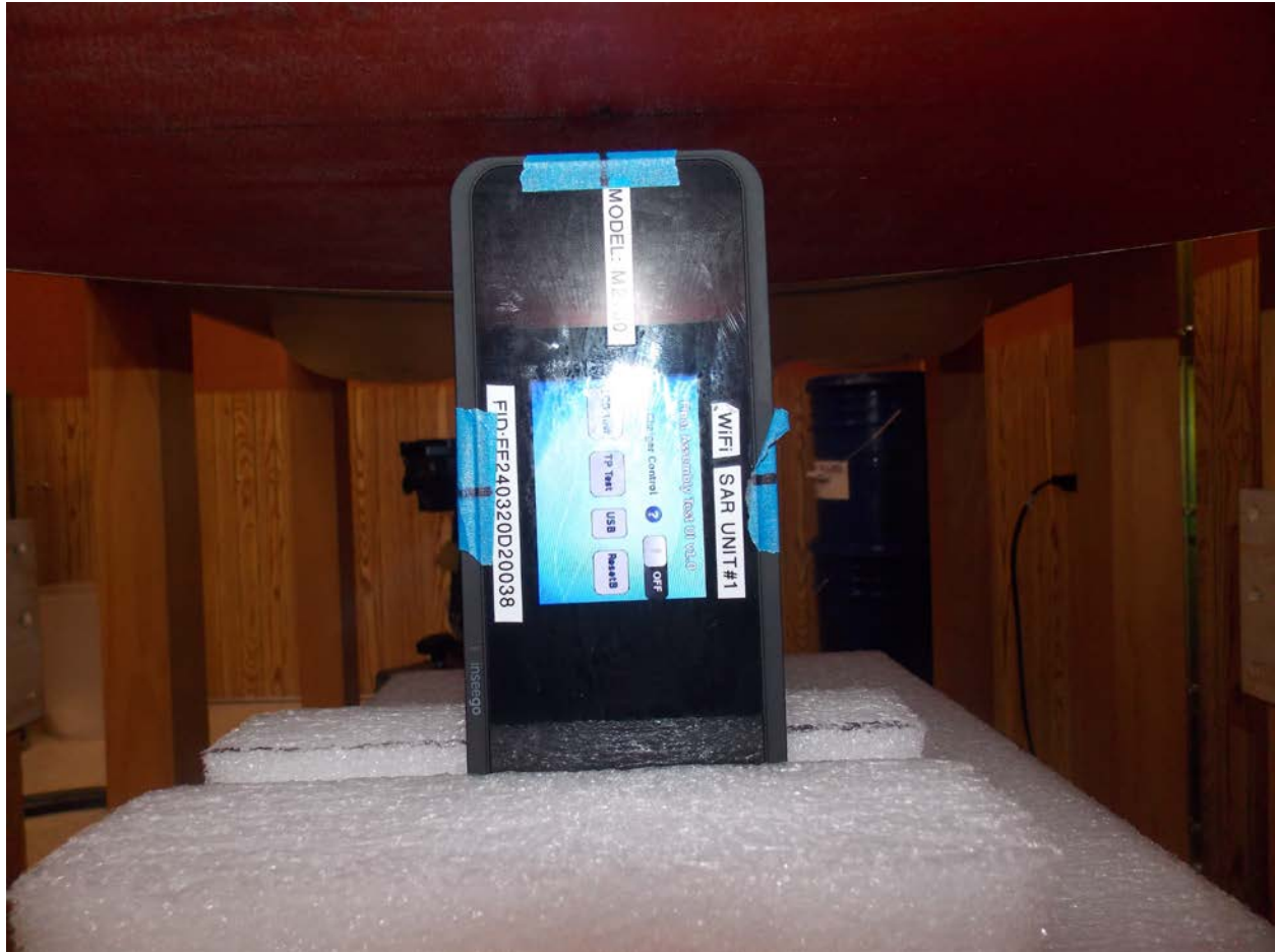
Test Position Side F 10 mm Gap
