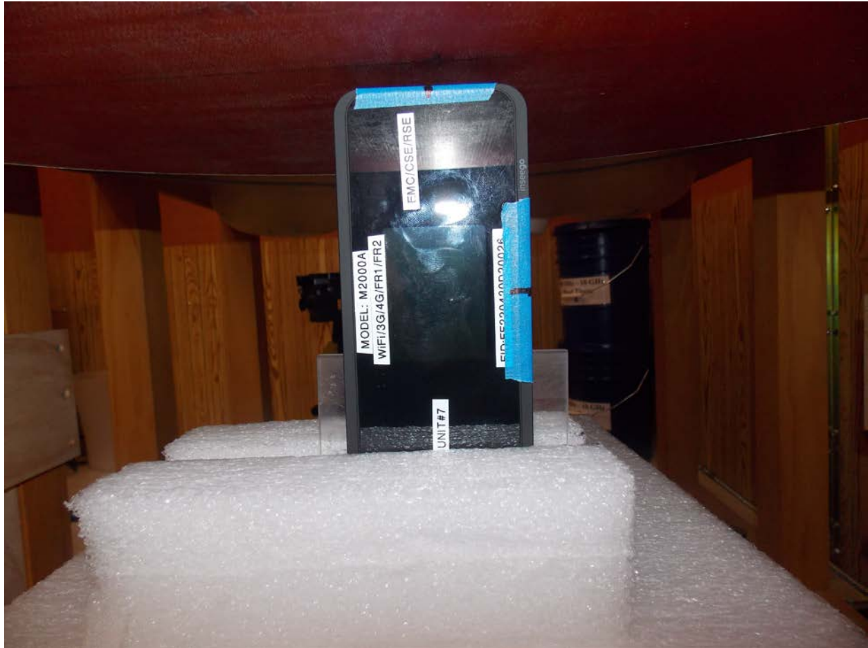
Test Position Side E 10 mm Gap
