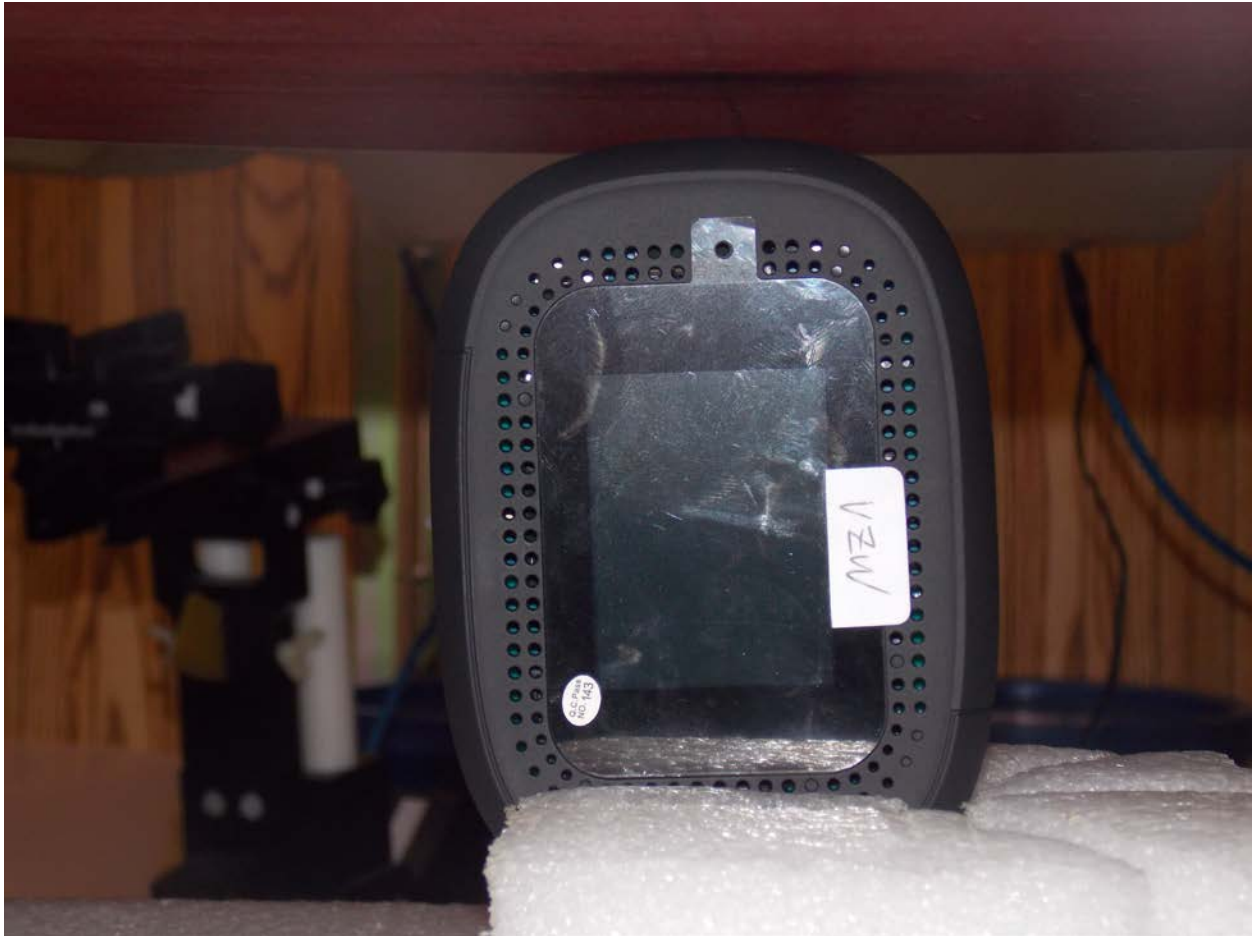
Test Position Side F 10 mm Gap
