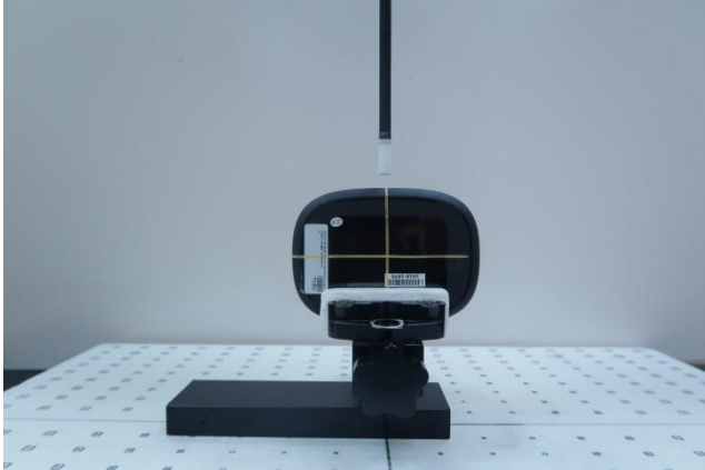
Front, Probe sensor to EUT surface distance 10mm
