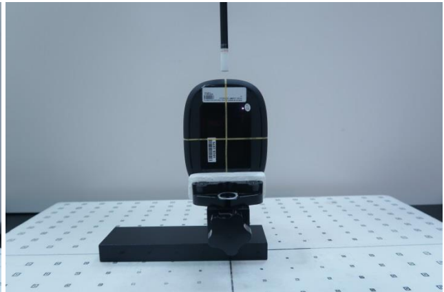
Right Side, Probe sensor to EUT surface distance 10mm
