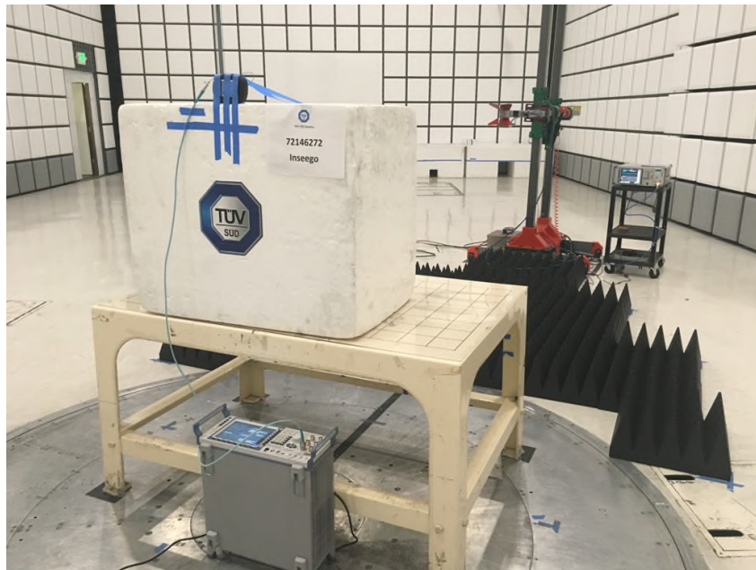
Radiated Emissions Above 1GHz Rear (Cell Transmission Mode)
