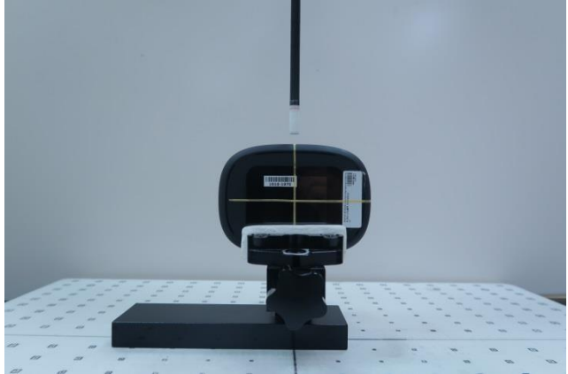
Back, Probe sensor to EUT surface distance 10mm
