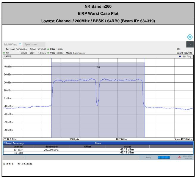
Offset = Antenna Factor (dB/m) + Cable Loss (dB) + 107 + 20log (D) - 104.8 = 43.8 + 2.72 + 107 + 20log(1.2) - 104.8 = 50.30 (dB)
