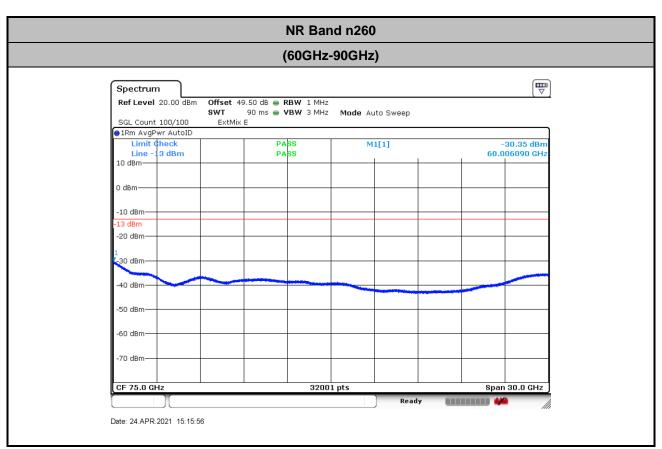
Offset = Antenna Factor (dB/m) + Cable Loss (dB) + 107 + 20log (D) - 104.8 = 45.4 + 0.34 + 107 + 20log(1.2) - 104.8 = 49.5 (dB)
