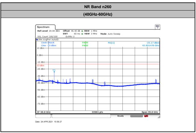
Offset = Antenna Factor (dB/m) + Cable Loss (dB) + 107 + 20log (D) - 104.8 = 42.3 + 0.34 + 107 + 20log(1.2) - 104.8 = 46.4 (dB)
