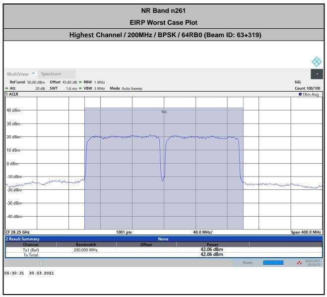
Offset = Antenna Factor (dB/m) + Cable Loss (dB) + 107 + 20log (D) - 104.8 = 39.4 + 2.65 + 107 + 20log(1.2) - 104.8 = 45.83 (dB)
