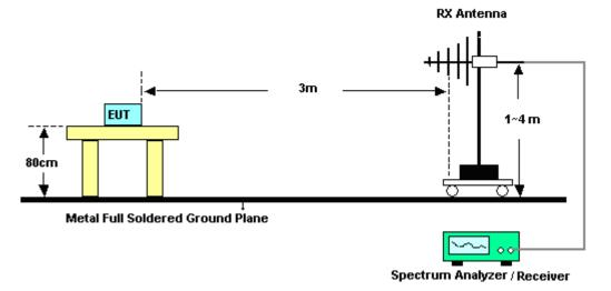
For radiated emissions 1GHz to 18GHz
