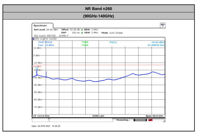
Offset = Antenna Factor (dB/m) + Cable Loss (dB) + 107 + 20log (D) - 104.8 = 48.8 + 0.34 + 107 + 20log(1.2) - 104.8 = 52.9 (dB)
