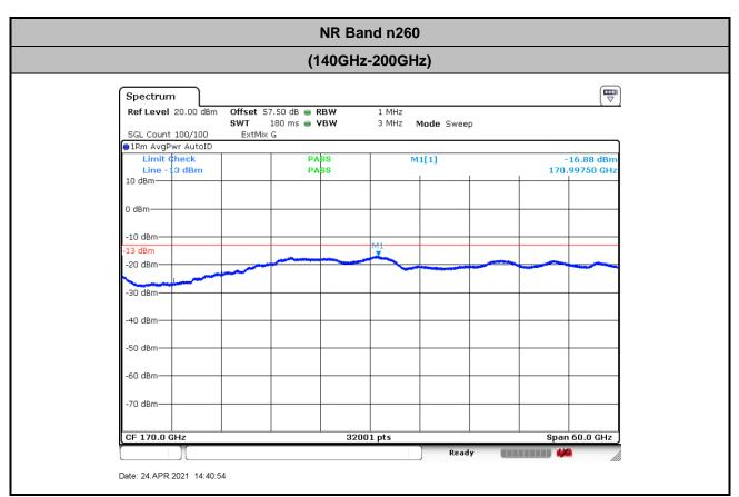
Offset = Antenna Factor (dB/m) + Cable Loss (dB) + 107 + 20log (D) - 104.8 = 53.4 + 0.34 + 107 + 20log(1.2) - 104.8 = 57.5 (dB)
