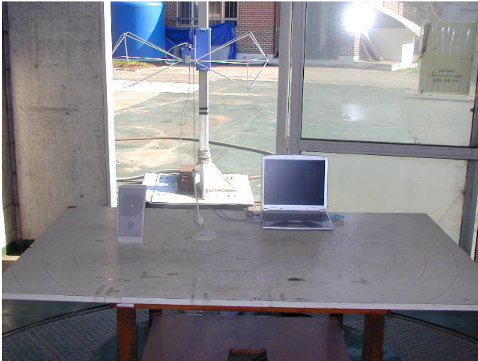
RADIATED EMISSION SETUP PHOTOGRAPH - FRONT VIEW ( 30 - 300 MHz )
