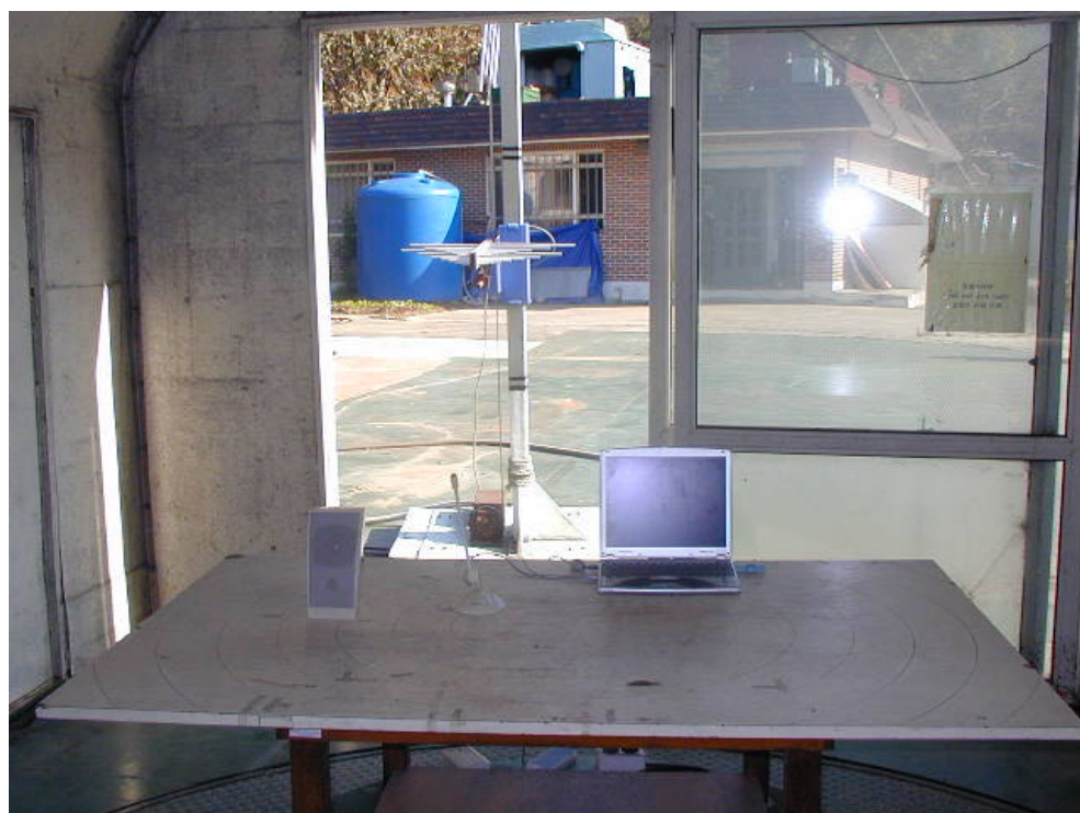
RADIATED EMISSION SETUP PHOTOGRAPH - FRONT VIEW ( 300- 1000 MHz )
