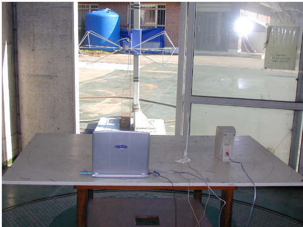
RADIATED EMISSION SETUP PHOTOGRAPH - REAR VIEW ( 30 - 300 MHz )
