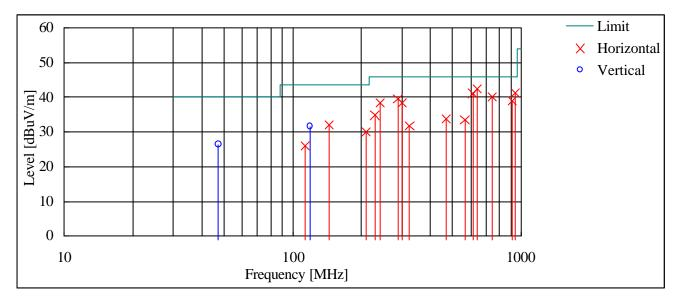
Notes: The test is performed in a distance of 3m. Af: Antenna factor, Cl: Cable loss
