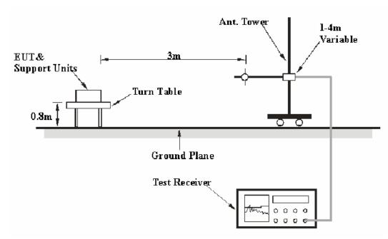
The radiated emission tests were performed in the 3 meters chamber B test site, using the setup accordance with the ANSI C63.4 - 2003. The specification used was the FCC 15 § 15.209 and 15.231.
