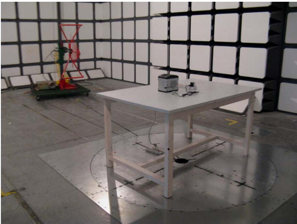
Radiated Emission - Rear View (Below 1GHz)
