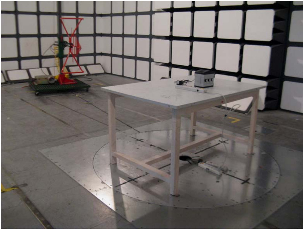
Radiated Emission - Rear View (Below 1GHz)
