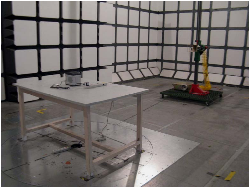
Radiated Emission - Rear View (Above 1GHz)
