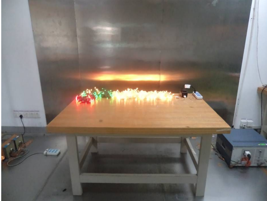
Conducted Emissions - Front View
