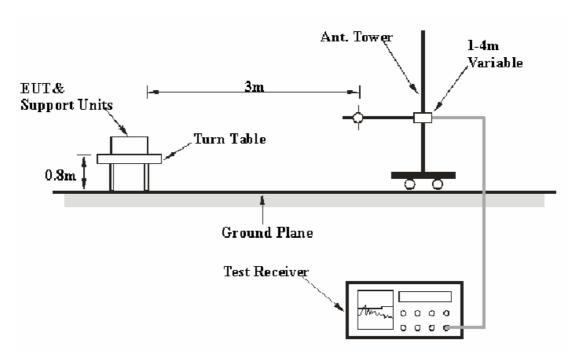
The deactivation test was performed in the 3 meters chamber B test site, using the setup accordance with the ANSI C63.4 - 2003. The specification used was the FCC 15.231(a) limits.
