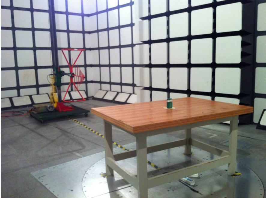
Radiated Emission View (Below 1 GHz)
