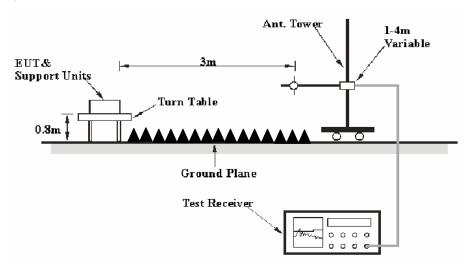
The radiated emission tests were performed in the 3 meters test site, using the setup accordance with the ANSI C63.4 - 2009. The specification used was the FCC 15 § 15.209, 15.205 and 15.231.
