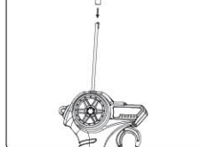
Diagram 2 ANTENNA TUBE INSTALLATION
