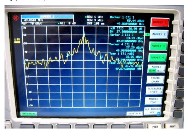
The results: The unit does meet the FCC Part 15 C Section 15.235 requirements.
