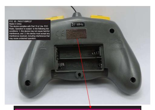
FCC ID: PKG17159RC27 Made in China This device complies with Part 15 of the FCC Rules, Operation is subject to the following two conditions: 1. this device may not cause harmful interference, and 2. this device must accept any interference received, including interference that may cause undesired operation.
