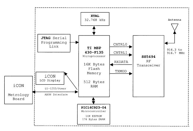
The TI MSP 430 series Microprocessor responds to commands received from the Site Controller via the SS5494 RF Transceiver. A "Read Status" command from the Site Controller results in the Microprocessor sending the current meter count to the Site Controller along with a Status Byte that reflects the value of its Retry Counter and Power failure notification.
