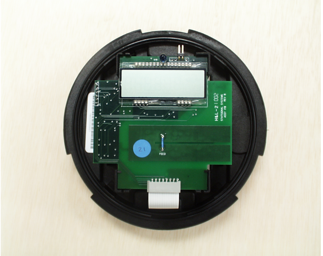
Internal Photograph 3: Top view of transmitter circuit board (assembled)
