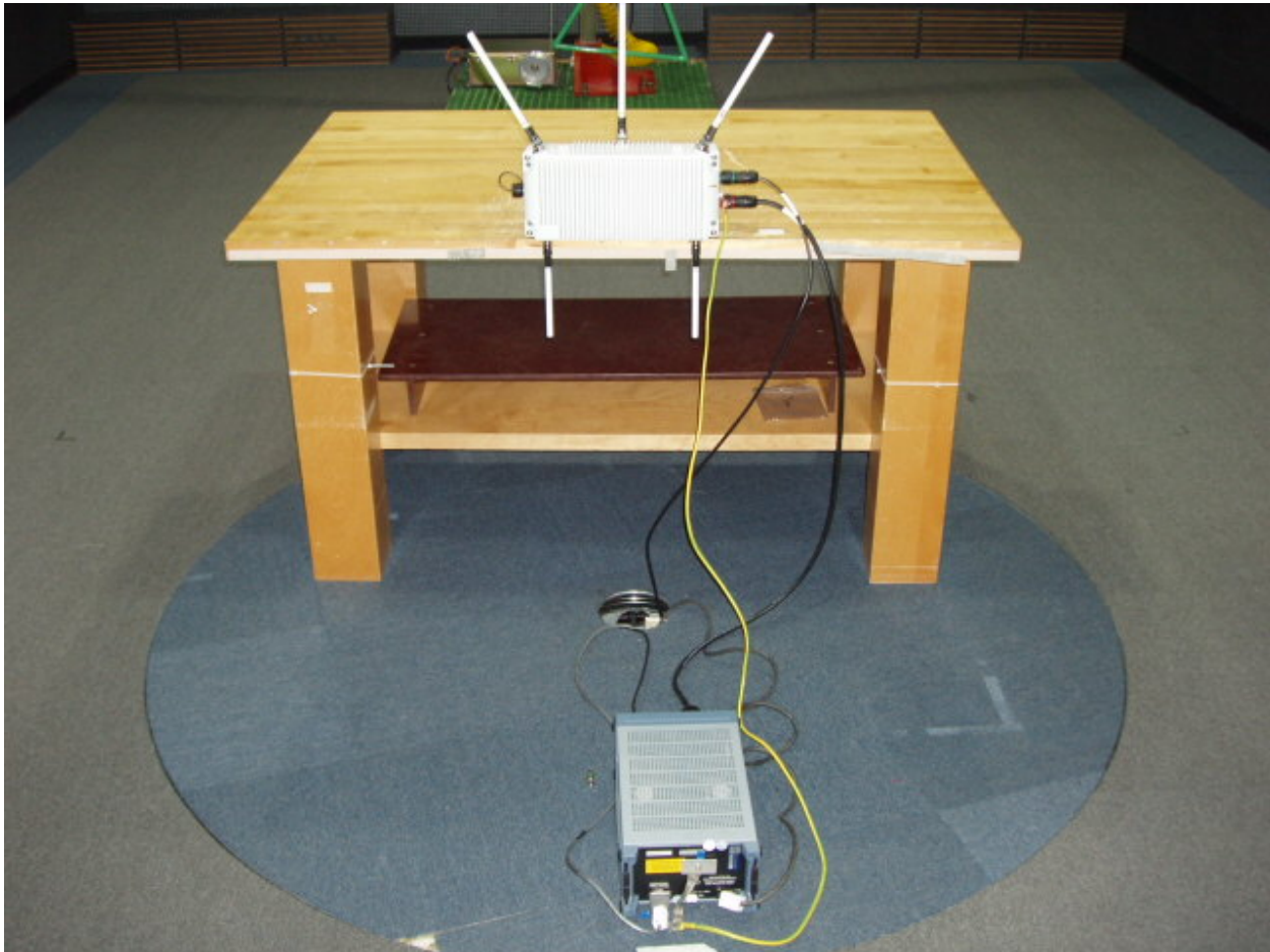
Photo 4.4-2 – Rear View of Conducted Emissions Test Set-up
