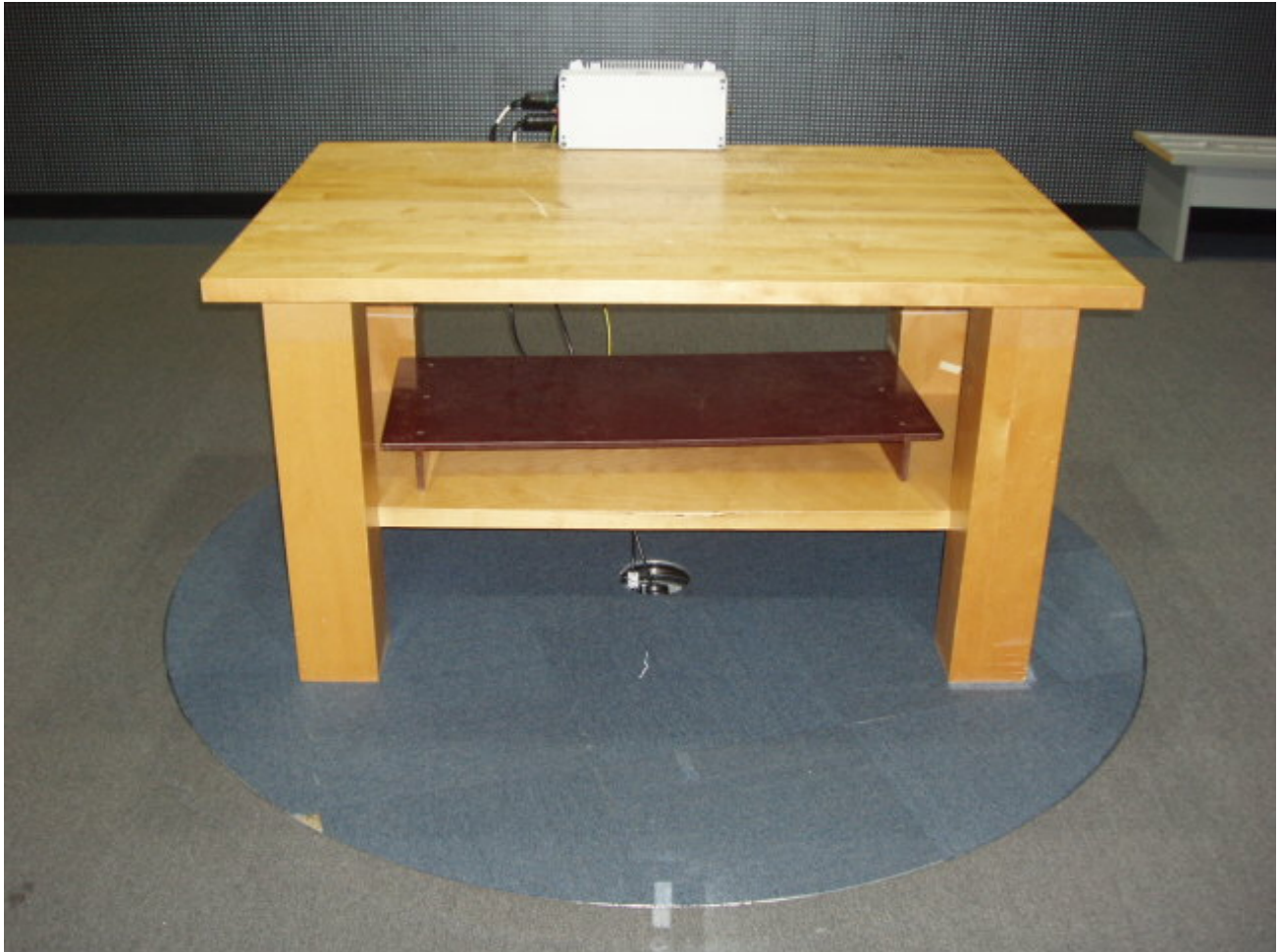
Photo 9.5-1 Front View of Radiated Emissions Test Set-up
