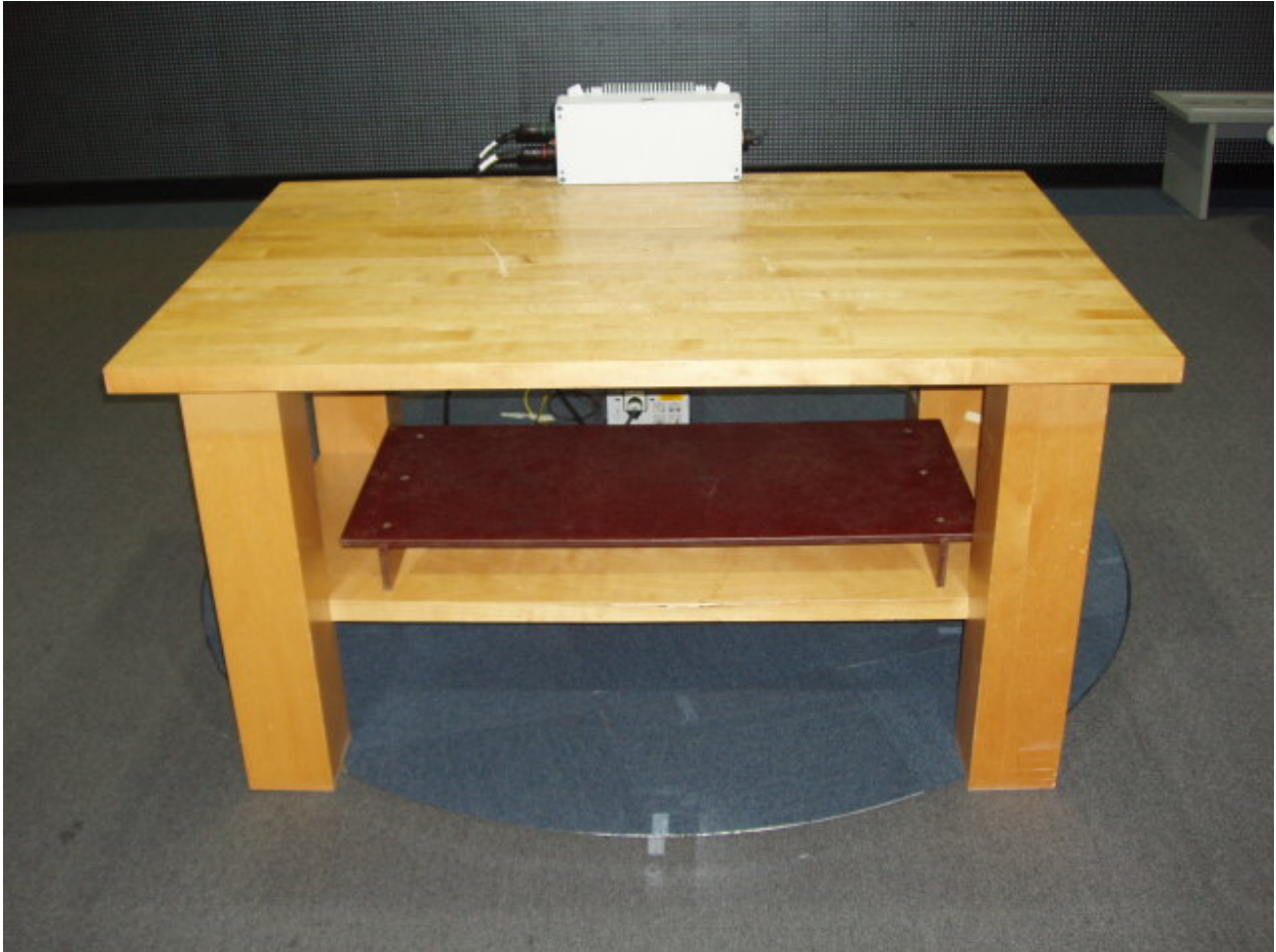
Photo 4.4-1 – Front View of Conducted Emissions Test Set-up
