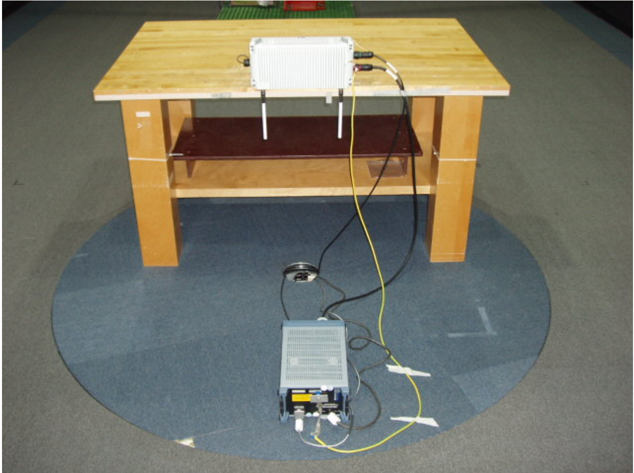
Photo 4.4-2 – Rear View of Conducted Emissions Test Set-up
