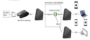
Example deployment where the main Gateway supports Wi-Fi and it supports a native MoCA 2.0 interface (or the MoCA 2.0 is implemented by an external bridge).
