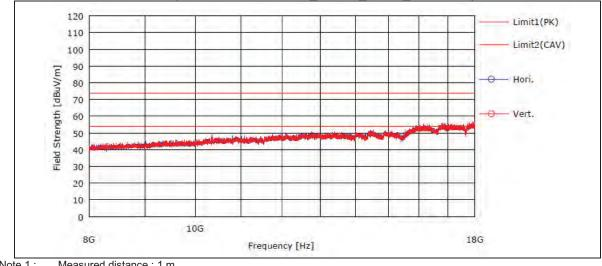
Test mode : 8 GHz ~ 18 GHz (Worst case : 802.11ac\_VHT80\_MIMO\_5775 MHz)
