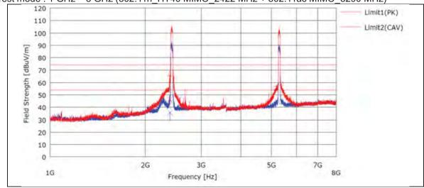
Test mode : 1 GHz ~ 8 GHz (802.11n HT40 MIMO 2422 MHz + 802.11ac MIMO 5290 MHz)
