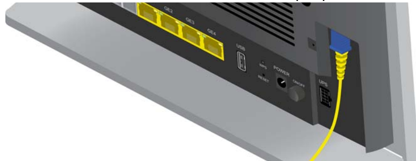
Figure 17: zNID-GE-27xx models use SC/UPC connector (blue)
