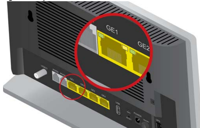
Figure 9: Log into GE port 1 to reach the Web UI or CLI on the zNID
