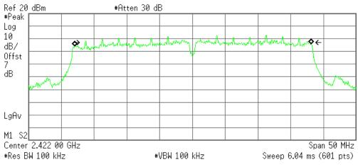
Occupied Bandwidth 35.9933 MHz Occ BW % Pwr 99.00 % x dB -6.00 dB
