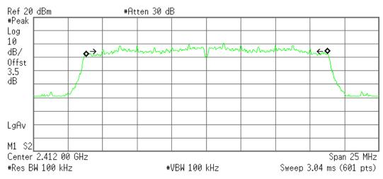
Occupied Bandwidth 17.4072 MHz Occ BW % Pwr 99.00 % x dB -6.00 dB
