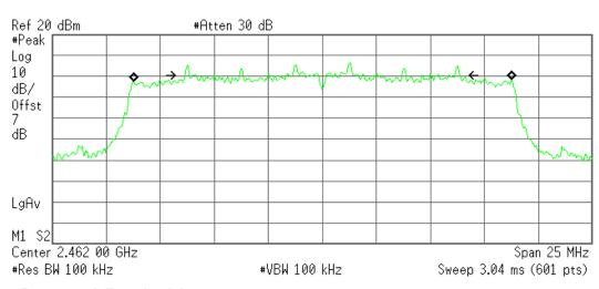
Occupied Bandwidth 17.4538 MHz Occ BW % Pwr 99.00 % x dB -6.00 dB
