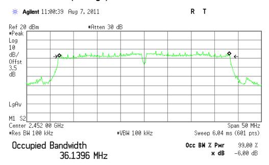
Transmit Freq Error 47.677 kHz x dB Bandwidth 35.795 MHz
