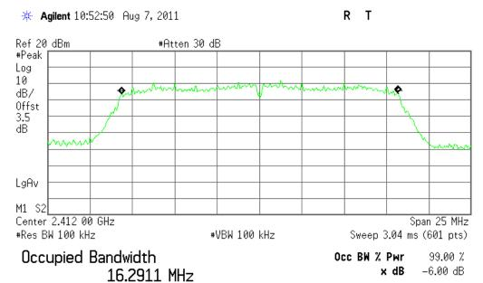
Transmit Freq Error 21.632 kHz x dB Bandwidth 15.130 MHz
