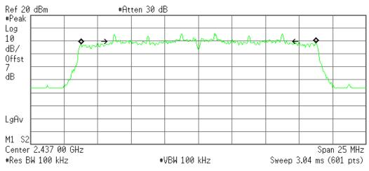
Occupied Bandwidth 17.4667 MHz Occ BW % Pwr 99.00 % x dB -6.00 dB
