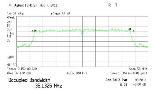
Transmit Freq Error 63.416 kHz x dB Bandwidth 36.015 MHz
