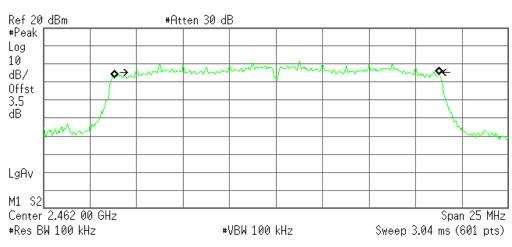
Occupied Bandwidth 17.4193 MHz Occ BW % Pwr 99.00 % x dB -6.00 dB
