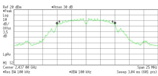
Occupied Bandwidth 10.0471 MHz Occ BW % Pwr 99.00 % × dB -6.00 dB
