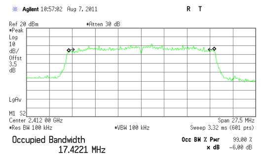
Transmit Freq Error 29.326 kHz x dB Bandwidth 15.112 MHz
