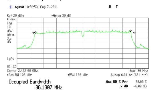
Transmit Freq Error 56.150 kHz x dB Bandwidth 35.810 MHz
