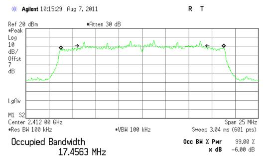
Transmit Freq Error 27.162 kHz x dB Bandwidth 12.743 MHz
