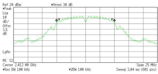
Occupied Bandwidth 10.0524 MHz Occ BW % Pwr 99.00 % x dB -6.00 dB
