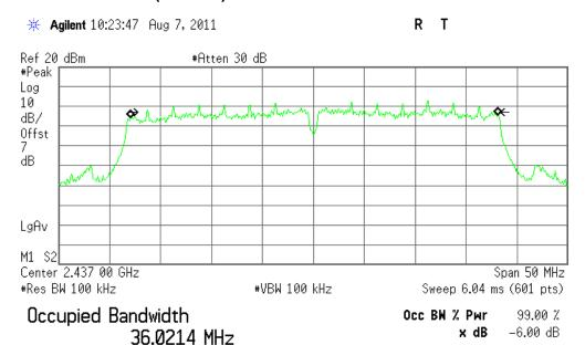
Transmit Freq Error 82.890 kHz x dB Bandwidth 33.847 MHz
