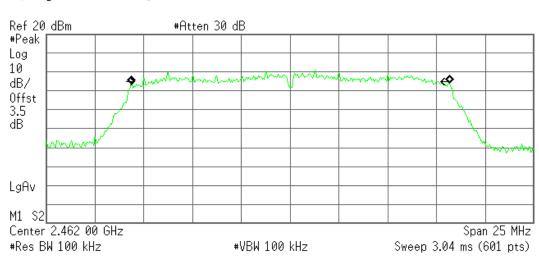
Occupied Bandwidth 16.2946 MHz Occ BW % Pwr 99.00 % x dB -6.00 dB
