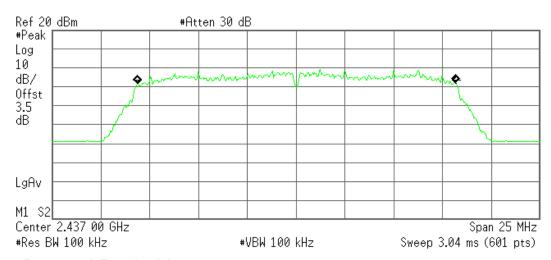
Occupied Bandwidth 16.2882 MHz Occ BW % Pwr 99.00 % x dB -6.00 dB
