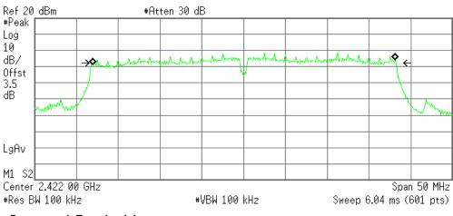
Occupied Bandwidth 36.1415 MHz Occ BW % Pwr 99.00 % x dB -6.00 dB
