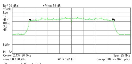
Occupied Bandwidth 17.4272 MHz Occ BW % Pwr 99.00 % x dB -6.00 dB
